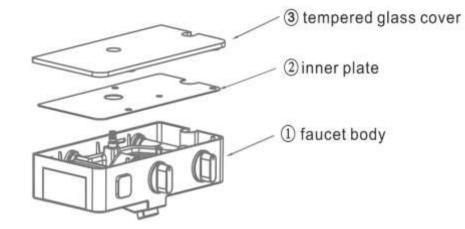
Step 4 Insert the faucet body into the brass connectors, tighten the hex nuts when the faucet body fits closely to the wall.
